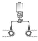
**Multiple point installation** is possible using a progressive distributor. Do not block any connections to the progressive distributor. Instead use a suitable distributor in accordance with the number of lubrication points. Keep the distance between the distributor and the lubri-cation unit as short as possible.
