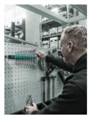
With its strong magnet, the rail can be attached securely to metal surfaces.
