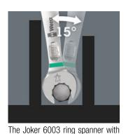
its special open end geometry - open end offset by 7.5° and the double hexagon profile - doubles the placement possibilities when repeatedly turning the wrench 180° around the longitudinal axis. Bolts and screw heads can be "accessed" every 15°. The Joker 6003 will automatically find the respective placement point after every turn.
