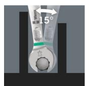
The Joker 6003 ring spanner with its special open end geometry open end offset by 7.5° and the double hexagon profile - doubles the placement possibilities when repeatedly turning the wrench 180° around the longitudinal axis. Bolts and screw heads can be "accessed" every 15°. The Joker 6003 will automatically find the respective placement point after every turn.
